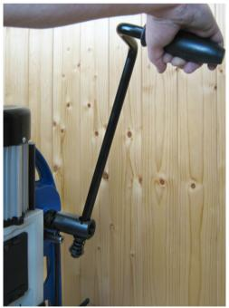
The starting position of the operating handle can be adjusted to a convenient and comfortable position.
