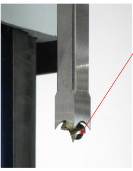
The Auger has a spur in the centre and a flat cutting lip. This cutting lip must be set below the four points of the chisel.
