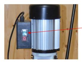
To start and stop the morticer, it is fitted with an NVR switch, located on the left hand side of the motor housing.
