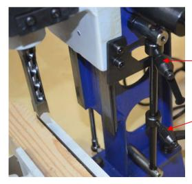
The top position (starting position) of the morticing head can be set by use of the upper stop. This is used to save time when working with smaller timber.
