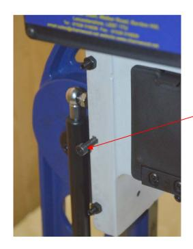
Locate the transport locking screw on the left hand side of the head. Loosen it using a 5mm hex key.
