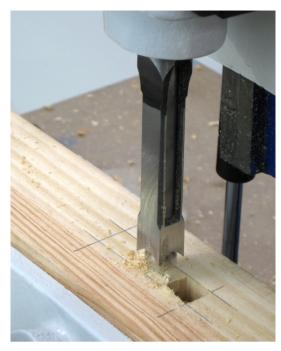
Start the motor, wait for it to come up to speed, pull down on the down feed handle of the morticer. You should aim for a cut rate that does not cause the motor to labour but still produces a progressive entry of the chisel into the wood.
