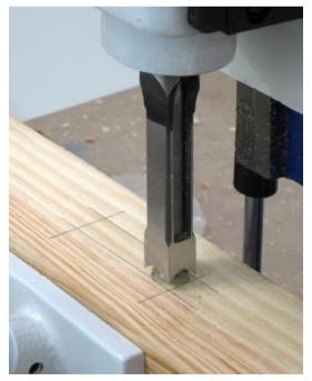
You may find it helpful to mark the outline of the mortice, including the depth, on the outside of the work piece. Set the depth limiter so that the points of the chisel reach the marked line. The tip will go below this line.
