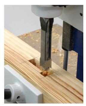
If the width of the mortice is bigger than the chisel being used:
