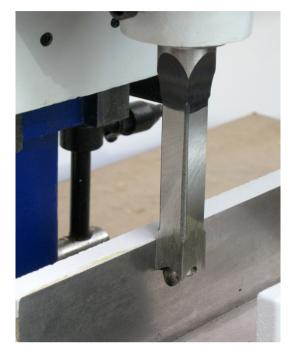
Next set the chisel square to the back fence. The easiest way to do this is to lower the chisel and wind the sliding bed forwards until it just touches the back of the chisel.
