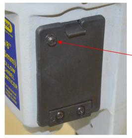
To gain access to the chuck for chisel and auger fitting or changing, you will need to loosen this screw (Ph2 head) and hinge the door downwards.
