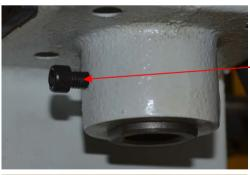
The chisel bushing is held in position by this set screw. It passes through the bushing and, when tightened, locks the chisel in place.
